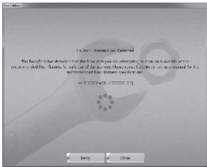
Figura 379: Pop-up Floor Validation Caution — Piso irregular detectado
